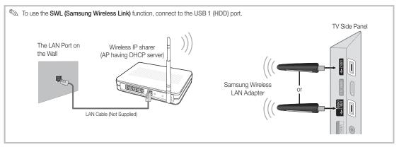
Samsung's Wireless LAN adapter is sold separately and is offered by select retailers, Ecommerce sites and Samsungparts. com. Samsung's Wireless LAN adapter supports the IEEE 802.11A/B/G and N communication protocols. Samsung recommends using IEEE 802.11N. When you play video over a IEEE 802.11B/G connection, the video may not play smoothly.
